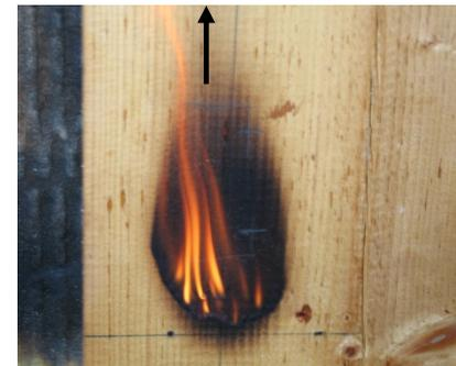
**Figure 1 Upward flame spread**
