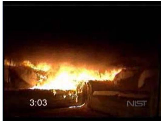
Pictures of fire development until flashover. Fire in a living room with plastic foam upholstered furniture (NIST). A door to the test hall was open.
